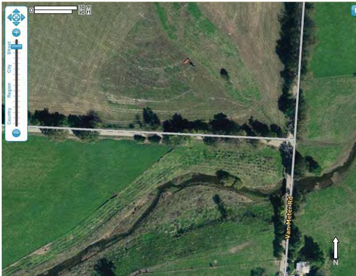
Figure 3.38: Lower reach of Hancock Creek, showing revegetated section with livestock exclusion fencing (center) and denuded banks with livestock access (right). Note variations in pasture grass density, a factor in sediment loading from sloped grazing areas. Source: Tetra Tech, 2008.
