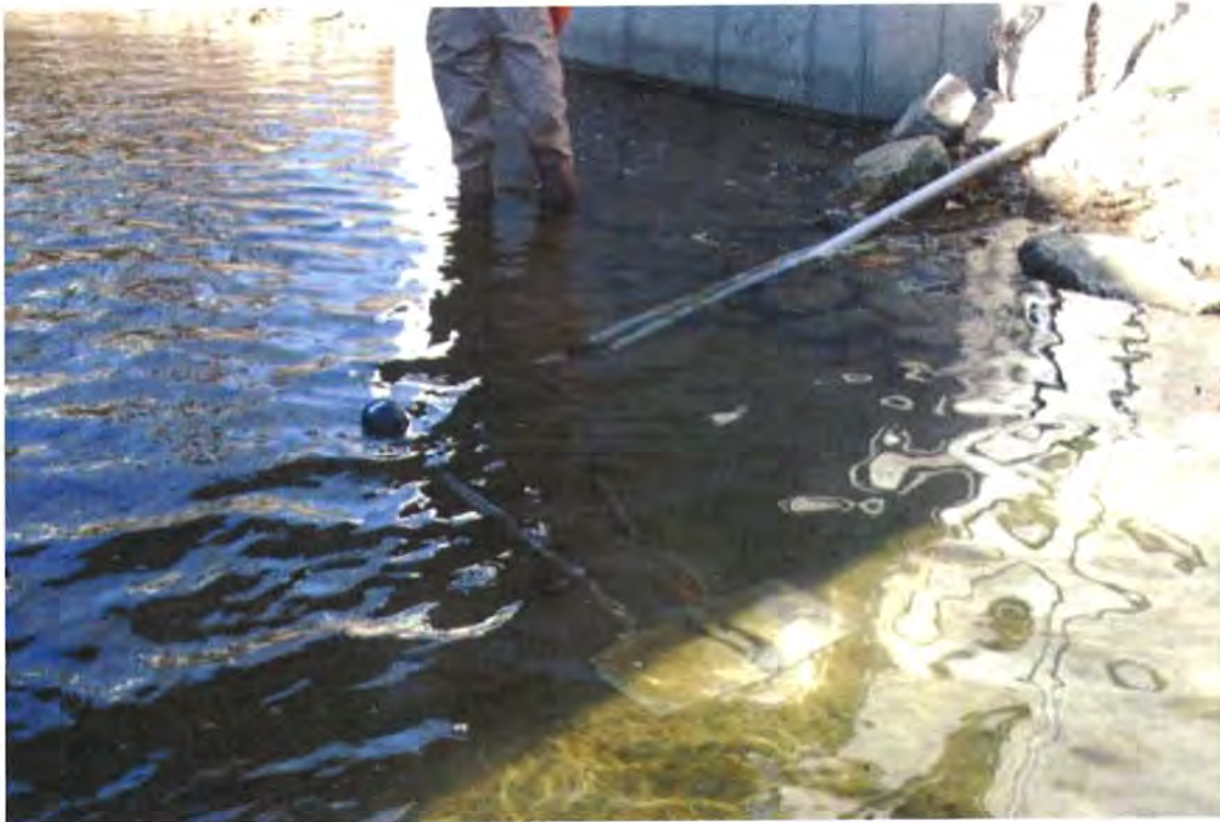
Figure 2.2 Typical ISCO set-up with intake on hinged rod.
