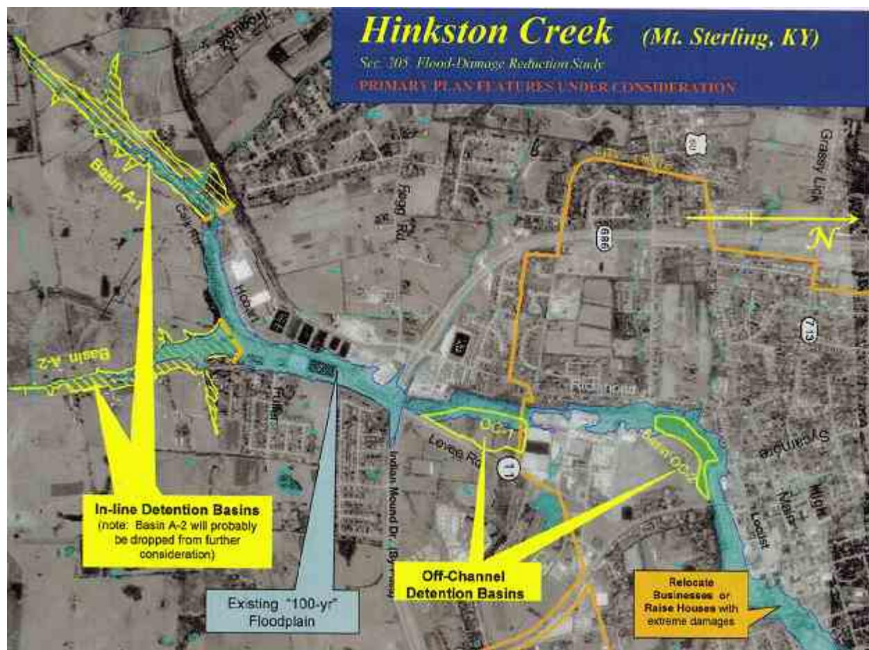
Figure 2-10. USACE Preliminary Detention Basin Plan for Upper Hinkston Creek in Mt. Sterling
